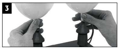
Place the balloon over the inflation outlet. Slightly roll the neck of the balloon over the tip. This will insure the gas enters the center of the balloon and the round shape of the balloon is maintained during the inflation process. It is important to inflate a test balloon at each adjustment until the desired size is produced.
