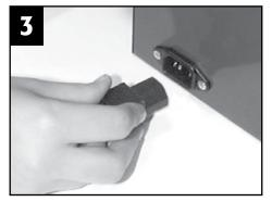
Plug the power cord into the back of the unit and into an electrical outlet. (A power strip with surge protector is recommened.) The digital display will appear when unit has power.
