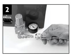
Push to connect the supply hose to the Speed Control Regulator on The Cube Inflator.
