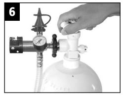
Slowly open the cylinder valve. Make sure the valve is fully opened. The cylinder pressure will read on the gauge located on the regulator. The inlet pressure will read on the Speed Control Regulator gauge, located on the back of the unit. Now the unit is ready to inflate balloons.
