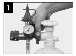
Hand-tighten the primary regulator to a helium or nitrogen cylinder. Make sure the cylinder is properly secured in a safety stand or wall bracket prior to attaching the primary regulator. Note: Do not open the cylinder valve until Step 6.
